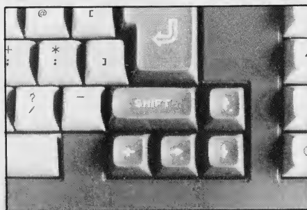
RETURN key is double size and cursor control keys are arranged reasonably.
